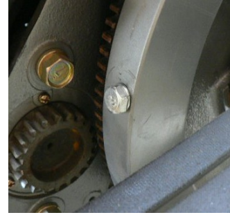
Trigger bolt installed on flywheel edge.
